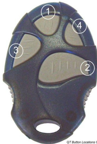
Figure 2: Button Configuration for Tag Programmed in “Standard Mode”
