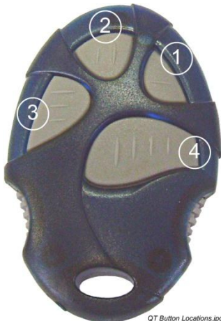
Figure 1: Button Configuration for Tag Programmed in “Dynamic Code Transmission Mode”
